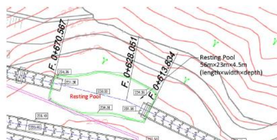
Figure 10: Fishway resting pool.
