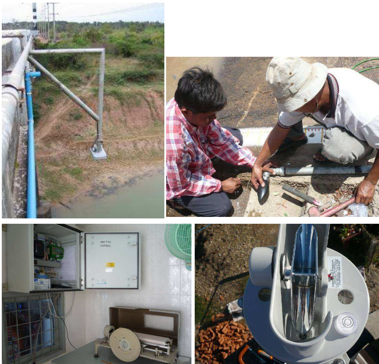
Figure 1 – Top Left: Radar water level sensor used at HYCOS stations; Top Right: Bubble river level sensor; Bottom Left: Shaft encoder and logging box; Bottom Right: Tipping bucket rain gauge. All photos from MRC (2012)
