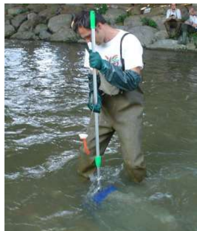
Figure 14 - Standard net for sampling (taken from AQEM sampling manual 2002).
