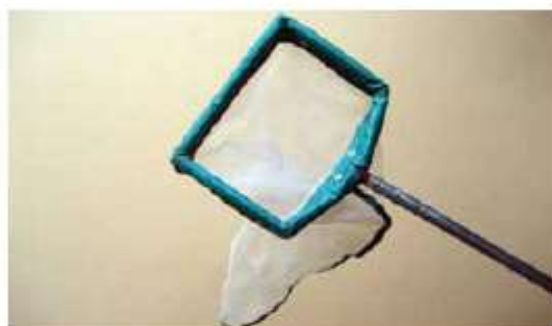
A D-frame net with 30cm x 20cm opening and mesh size of 475µm is used for sampling.
