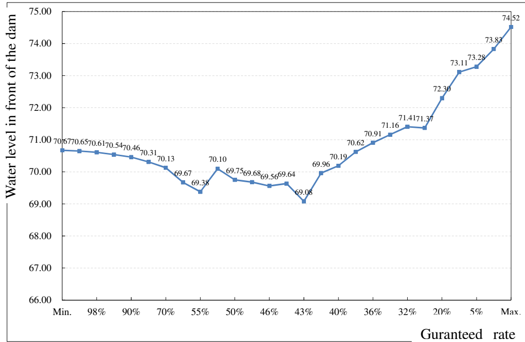
Figure 6.1-1 Process of Water level Changes in front of Dam under Inflows with Different guarantee rates (after the Modification project is put into operation)
