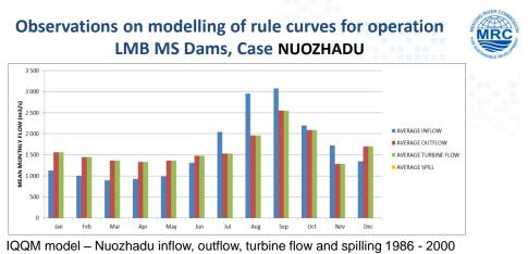
According to this figure there is no spilling. For the period January to July the reservoir water level is drawn down by 12 to 33 m, say in average 22 m, which represents about 10% headloss in relation to the max head of 210 m during the 6 months.
