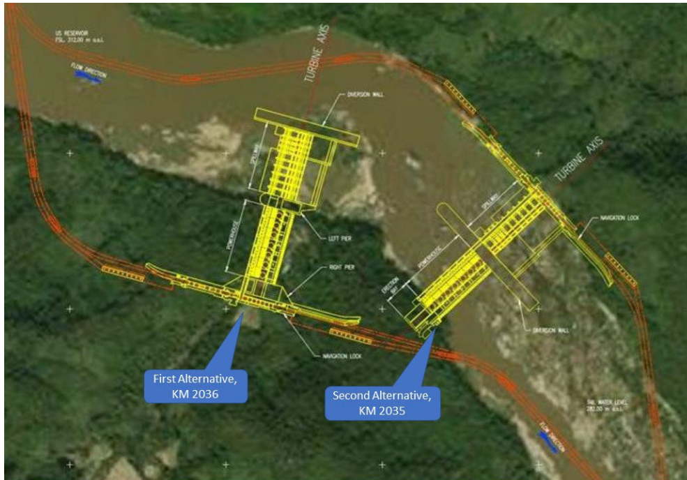
Figure 7: Overview of the two Sites for the Barrage
